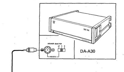
When using this unit with its companion power amplifier (DA-A30), make the connection between them as shown in the diagram.
